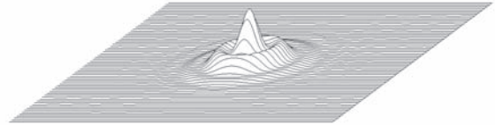
Figure 2. Uncorrected spherical aberrations lead to blurry focal spots. This illustration shows the point-spread function of a lens with spherical aberration at marginal focus.
